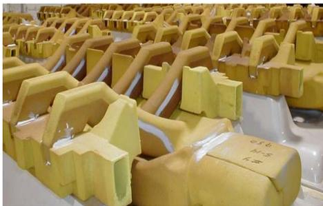
Shell molding, also known as shell-mold casting is an expendable mold casting process that uses a resin covered sand to form the mold. As compared to sand casting, this process has better dimensional accuracy, a higher productivity rate, and lower labor requirements. It is used for small to medium parts that require high precision.
